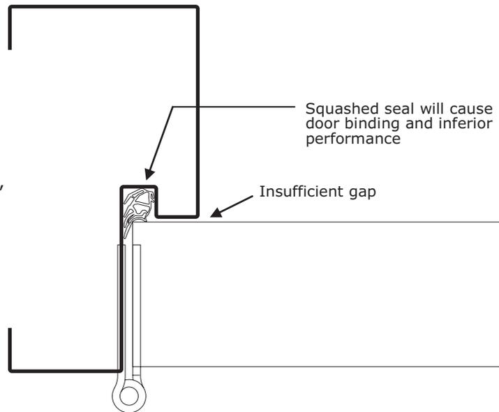
**NOTE: Correct closer selection is important for ALL doors fitted with compression seals. (If in doubt, please contact your hardware supplier to determine suitability)**
