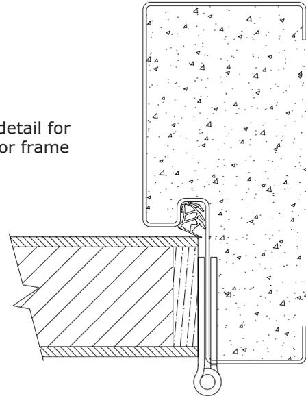
Typical detail for timber door frame
