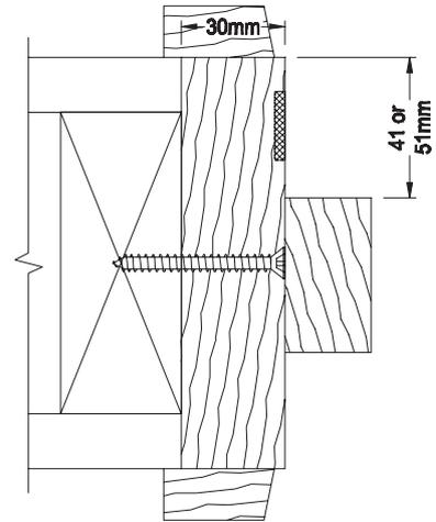
Typical frame profile - note hidden frame fixings
